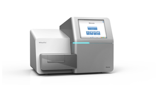
Figure 1: Illumina MiSeq FGx Instrument —The Illumina MiSeq FGx instrument is a compact, fully validated next-generation sequencing platform for forensic genomics applications.
